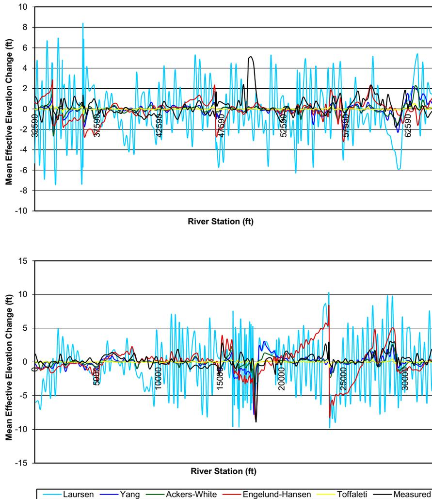
FIGURE 5. Averaged Bed Elevation Change from HEC-RAS Model.
