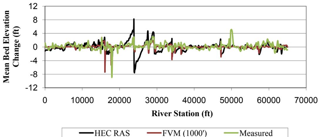
FIGURE 9. Comparison of Results from FVM and HEC-RAS Model (Engelund and Hansen's Method).
