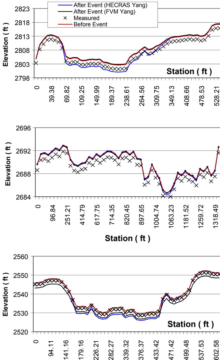
FIGURE 8. Samples of Cross-Section Changes Using HEC-RAS and FVM 1D Model.
