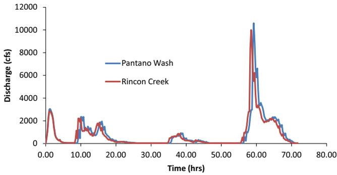
FIGURE 2. HEC-RAS Input Hydrograph at the Pantano Wash and Rincon Creek.
