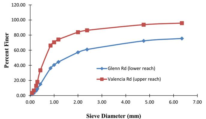
FIGURE 3. Bed Sediment Gradation Curve for Pantano Wash.
