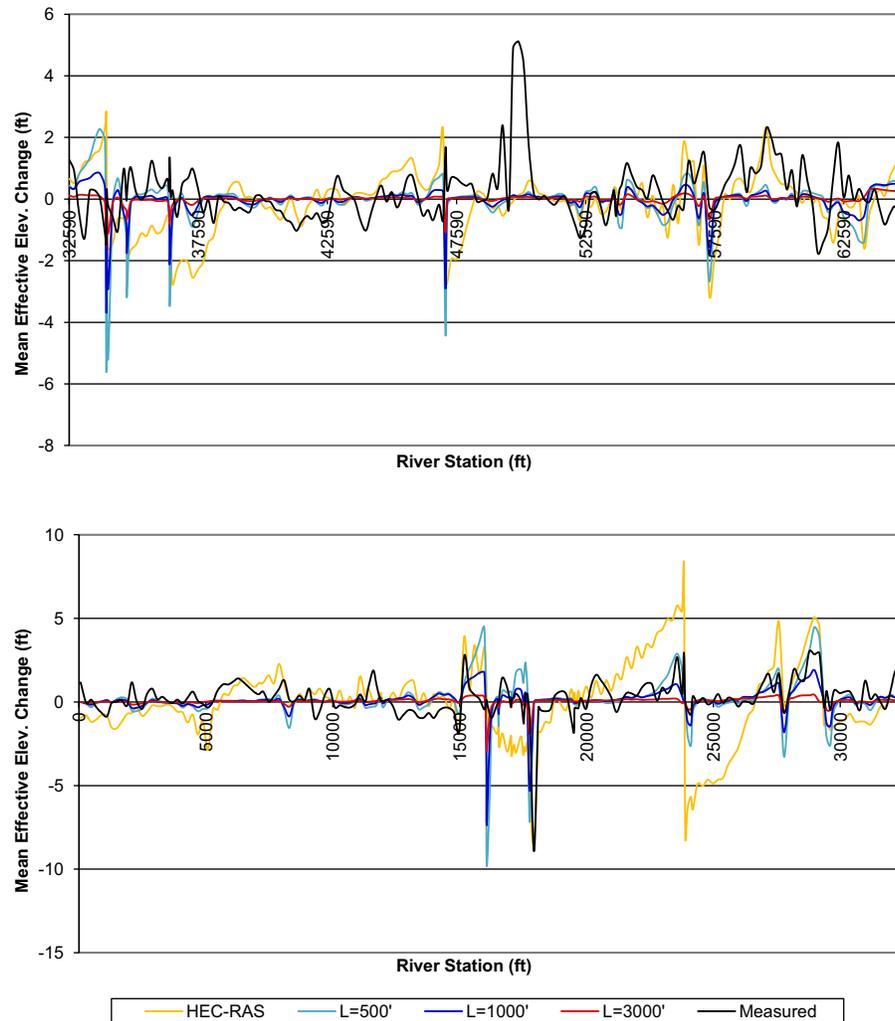
FIGURE 7. Comparison of the Results of FVM Model Using Engelund-Hansen's Transport Method.
