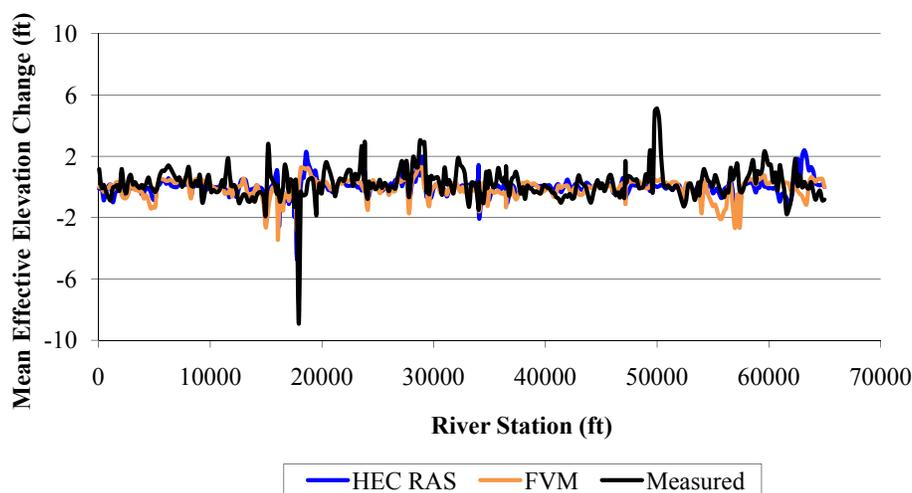
FIGURE 10. Comparison of Results from FVM and HEC-RAS Model (Yang's Method).
